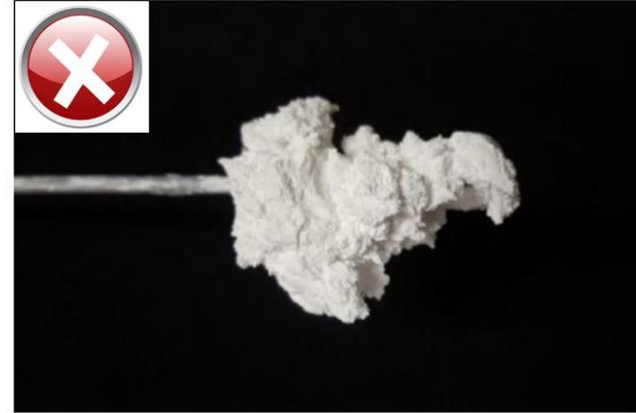
Heterogeneous paste resulting from directly mixing 90% solids
