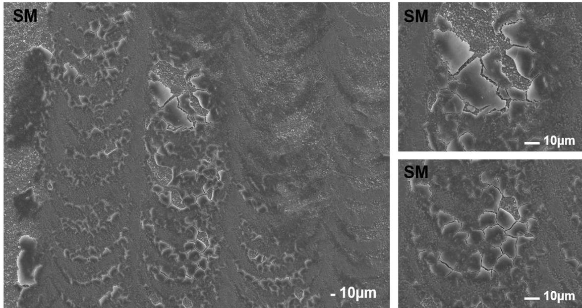
**Thick layer of adhered dental material, which covers almost all the tested area during chewing simulation**
