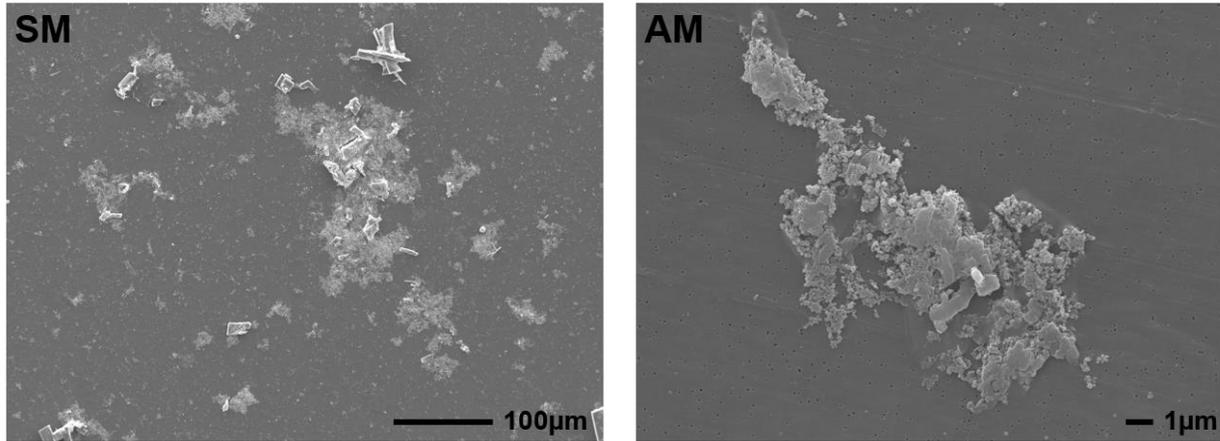
SM and AM filtered worn particles from the artificial saliva solution after wear testing
