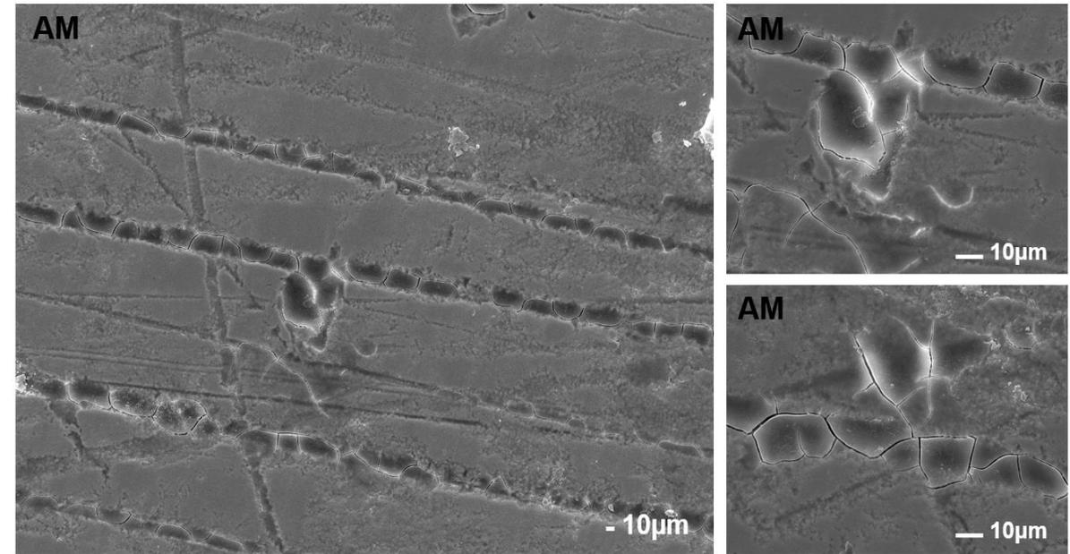
**AM samples present some scratches over the surface in which the worn dental particles adhered**
